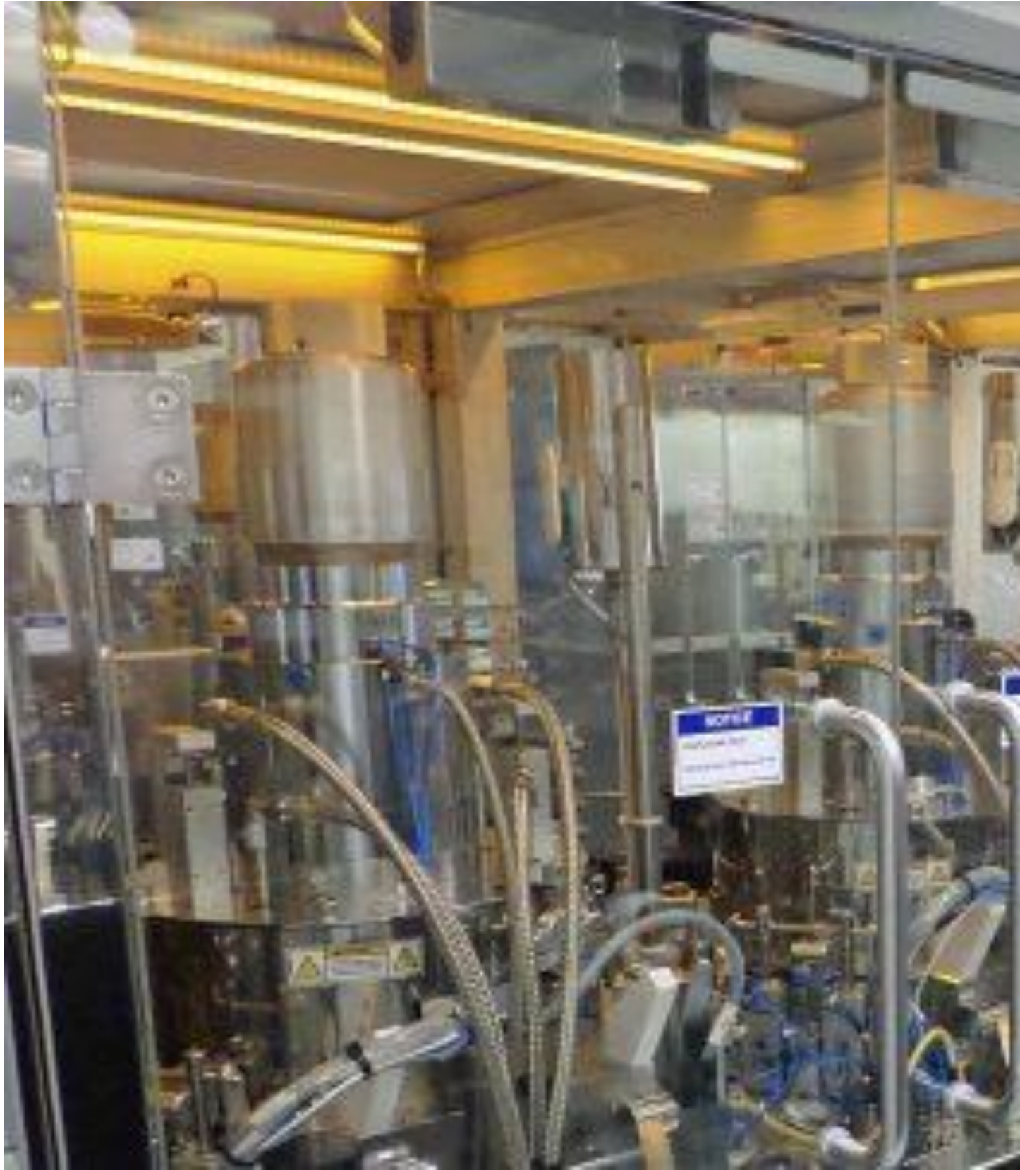
Fig. 4: Gemini Cluster Process tool for wafer-to-wafer bonding. Silicon wafer bonders and
